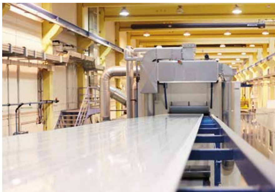
Continuous sandwich panel manufacturing with the most advanced and largest double conveyor belt production line in the world
