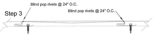
Use the supplied blind pop rivets to secure the panel cover to the damages panels face. Attach the blind pop rivets to each side of the panel at 24" O.C. Use the supplied textured touch-up paint to cover the blind pop rivets.
