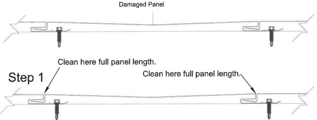
Using a brush or an air gun remove as much of the overspray from the 2 vertical edges (Bottom to top). Be Sure to protect the surface of the adjacent panels when cleaning out the overspray.
